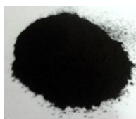
Fig. 1. The amino-MNPs powder prepared through polyol technique at 105 kPa, 121 °C, 2 hr per cycle for 3 cycles
