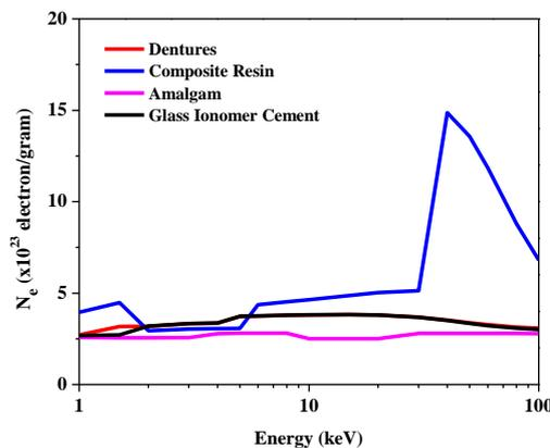
**Fig. 4** Effective electron densities of all dental materials versus photon energy range 1 keV–100 keV.
