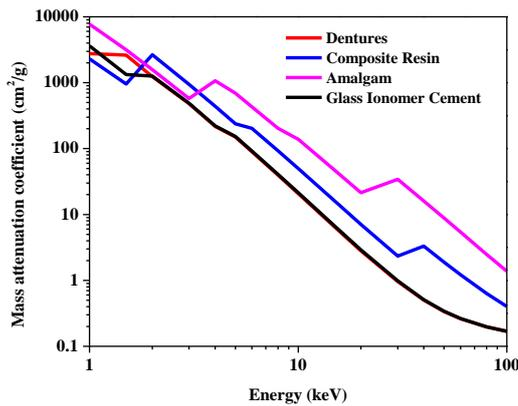
**Fig. 1** Mass attenuation coefficient of all dental materials versus photon energy range 1 keV–100 keV.
