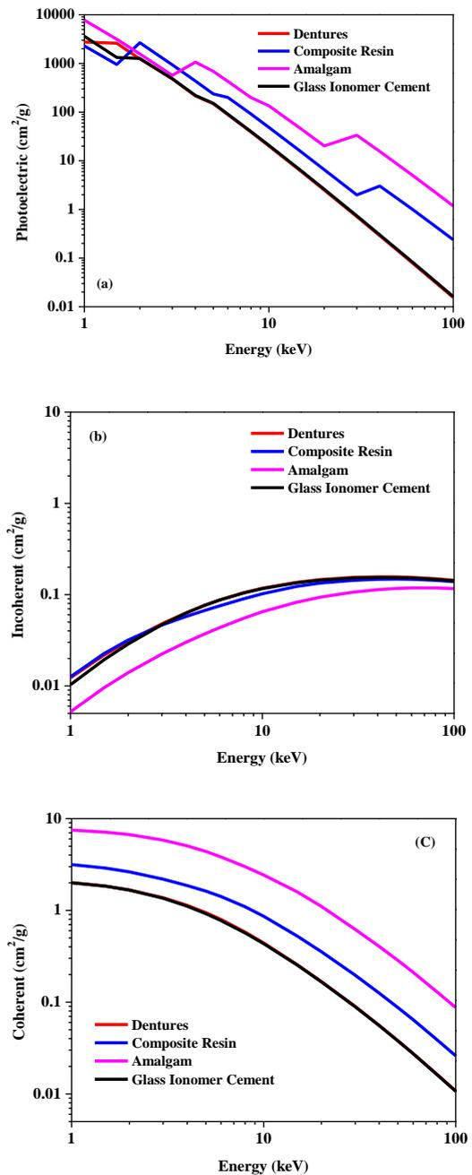
**Fig. 2** Partial interaction (a) photoelectric (b) incoherent (c) coherent, of all dental materials versus photon energy range 1 keV–100 keV.
