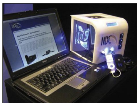
Fig. 1 Direct ethanol fuel cell, DEFC [9].
