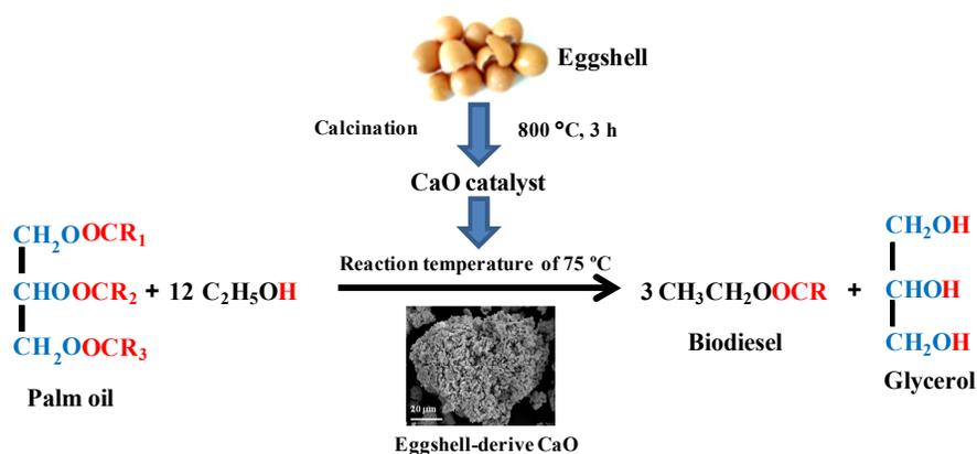
**Fig. 1** Flow diagram of the experiments for biodiesel synthesis by ethanolysis using CaO obtained from eggshell.
