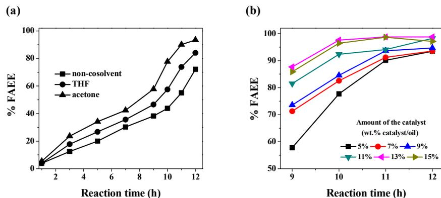
**Fig. 5** (a) %FAEE of with and without % v/v of co-solvent systems; reaction condition: catalyst amount of 5 wt.%, ethanol/oil molar ratio of 12:1 and reaction temperature of  $75\pm 2$  °C. (b) Effect of catalyst loading amount of % FAEE yield; reaction condition: 10% v/v acetone as a co-solvent system, ethanol/oil molar ratio of 12:1 and reaction temperature of  $75\pm 2$  °C.
