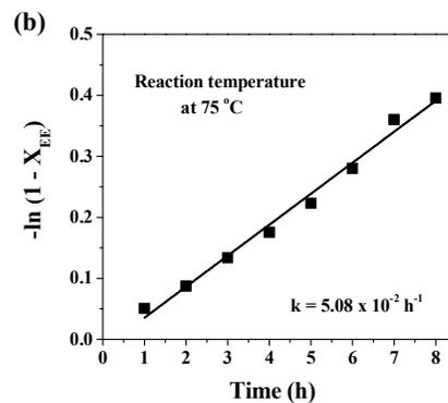
Fig. 4 (a) and (b) kinetics study of reaction. Reaction condition: catalyst amount of 5 wt.%, alcohol/oil molar ratio of 12:1, reaction temperature of  $65 \pm 2 \text{ }^\circ\text{C}$  using methanol and  $75 \pm 2 \text{ }^\circ\text{C}$  using ethanol.
