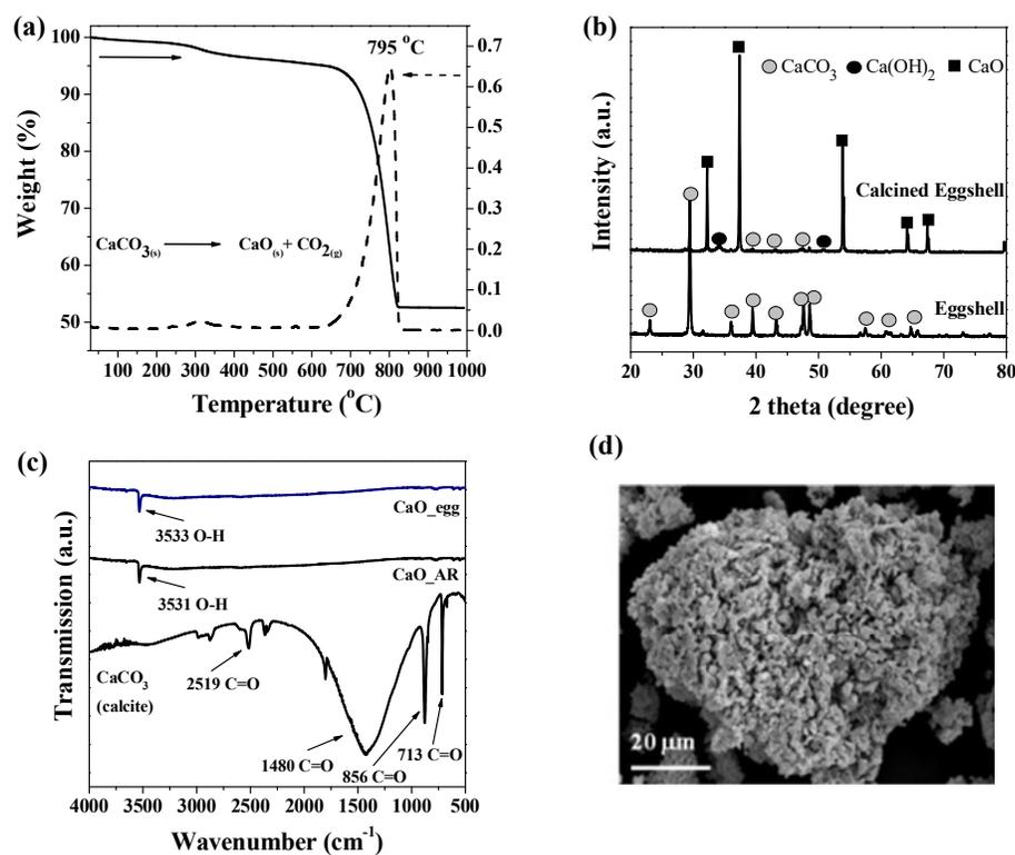
**Fig. 2** (a) TG/DTA thermograms of eggshell, (b) XRD patterns and (c) IR spectra of eggshell and eggshell calcined at 800 °C for 3 h and (d) SEM images of the eggshell calcined at 800 °C for 3 h.
