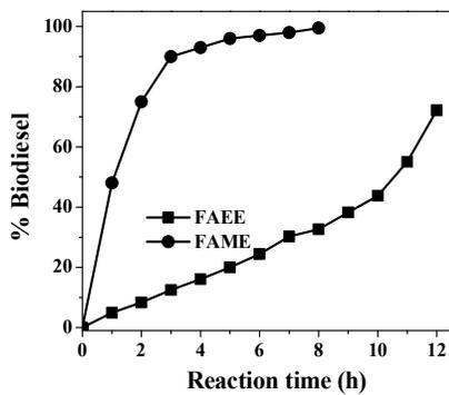
Fig. 3 Comparison of the effects of reagent between methanol and ethanol on biodiesel product.
