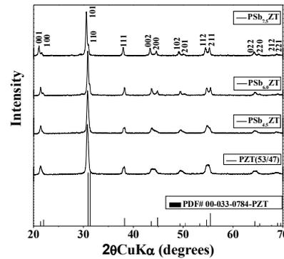
**Fig. 1** XRD pattern of PSbZT ceramics were sintered at 1,423 K for 2 h
