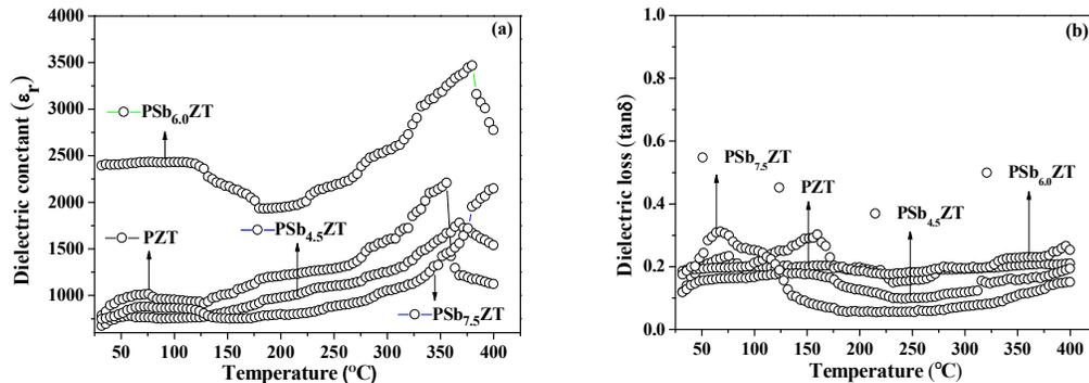
**Fig. 2** The relative dielectric constant (a) and dielectric loss (b) at the function of temperature and frequency 1 kHz. of PSbZT ceramics.
