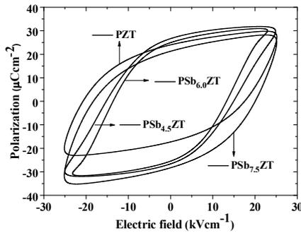
**Fig. 3** Room temperature P – E hysteresis loops of the PSbZT ceramics at electric field of  $25 \text{ kVcm}^{-1}$  and the frequency of 100 Hz.
