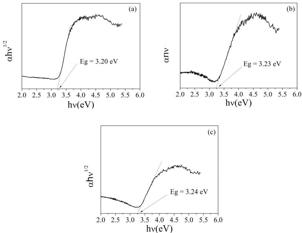
**Fig. 4** The determination of optical band gaps by the absorption as a function of light energy for titania nanotubes after hydrothermal process in different solutions: (a) acid, (b) neutral, and (c) base.
