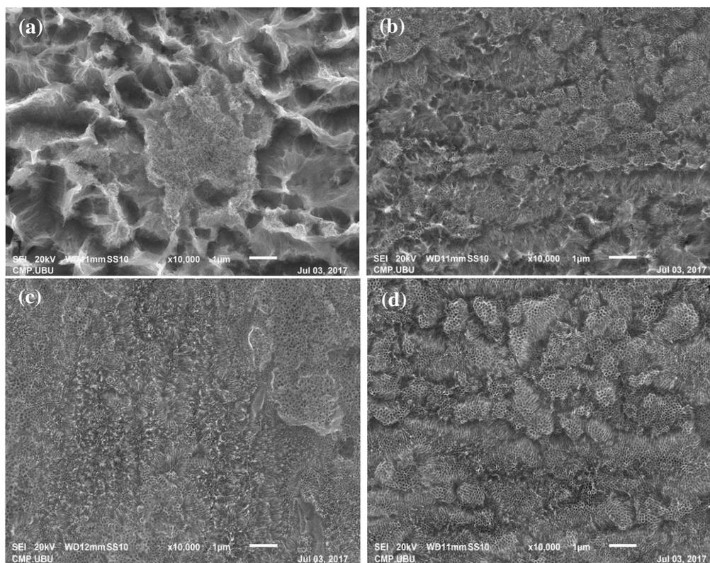
**Fig. 3** SEM images of titania nanotubes after anodization followed by different ultrasonic cleaning with different periods of time: (a) 0 min, (b) 10 min, (c) 30 min, and (d) 50 min.
