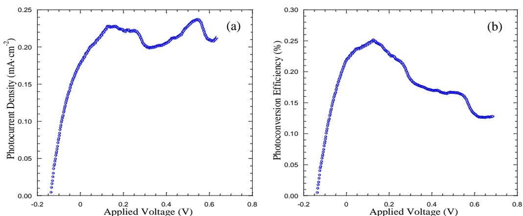
**Fig. 7** Performance of the photoelectrochemical cells for hydrogen production with photoanode of hydrothermal titania nanotubes treated with base solution (a) IV curve and (b) photoconversion efficiency as a function of an applied voltage.
