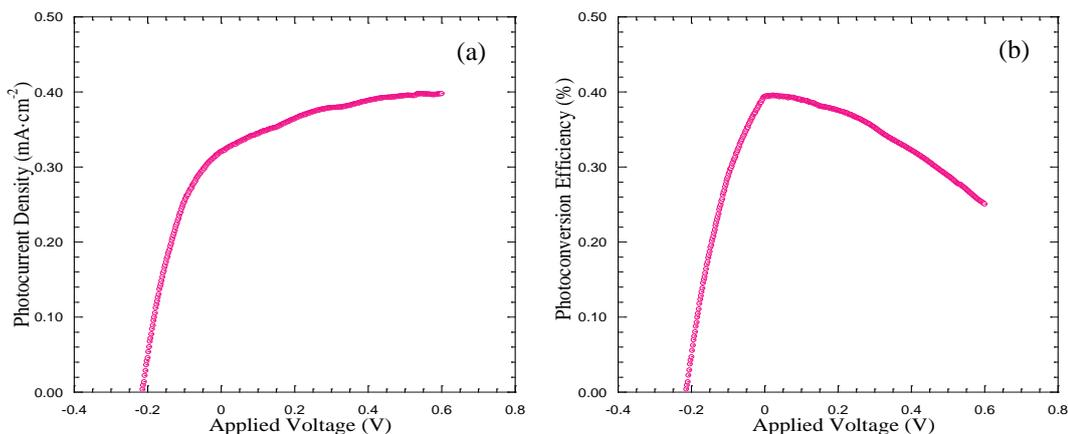
**Fig. 6** Performance of the photoelectrochemical cells for hydrogen production with photoanode of hydrothermal titania nanotubes treated with acid solution (a) IV curve and (b) photoconversion efficiency as a function of an applied voltage.
