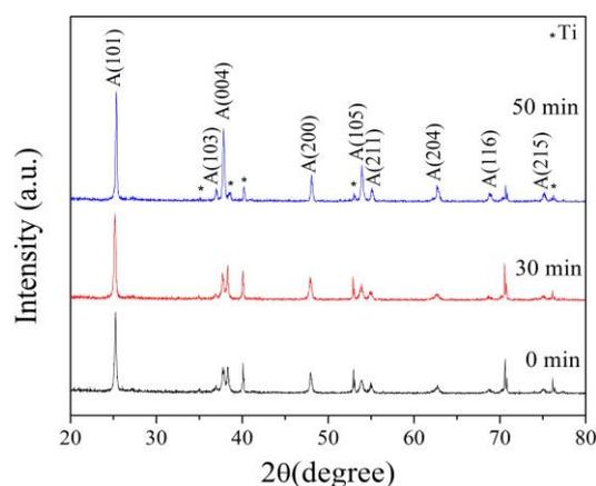
**Fig. 2** The XRD patterns of titania nanotubes with different cleaning time.
