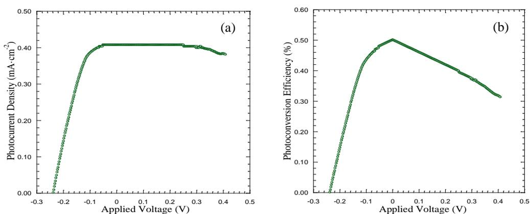
**Fig. 5** Performance of the photoelectrochemical cells for hydrogen production with photoanode of hydrothermal titania nanotubes treated with neutral solution (a) IV curve and (b) Photoconversion efficiency as a function of an applied voltage.
