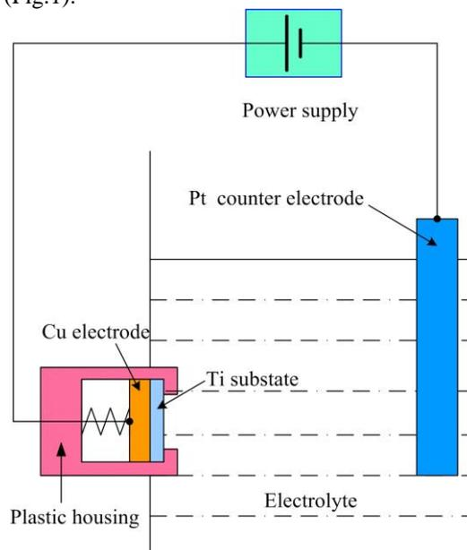
**Fig. 1** Experimental equipment diagram of one-face anodization for titania nanotubes [8]
